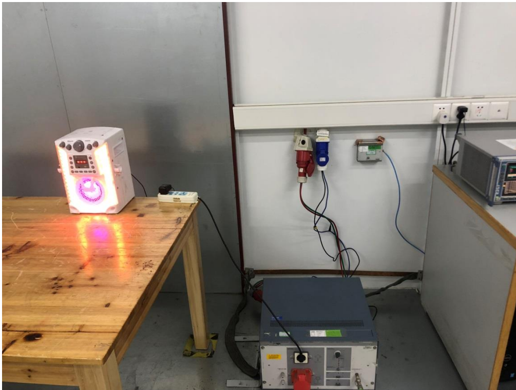
The adapter GKYZA0150058US RADIATED EMISSION TEST SETUP BELOW 1GHz
