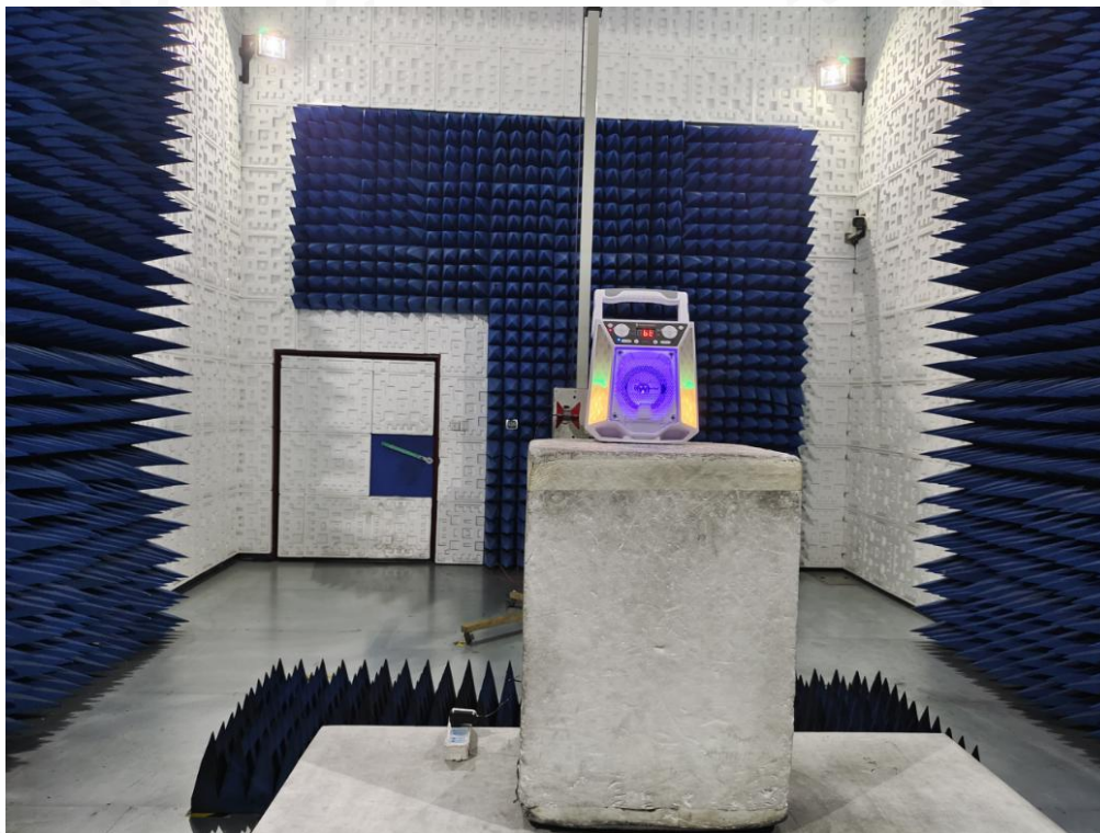
RADIATED EMISSION TEST SETUP ABOVE 1GHz
