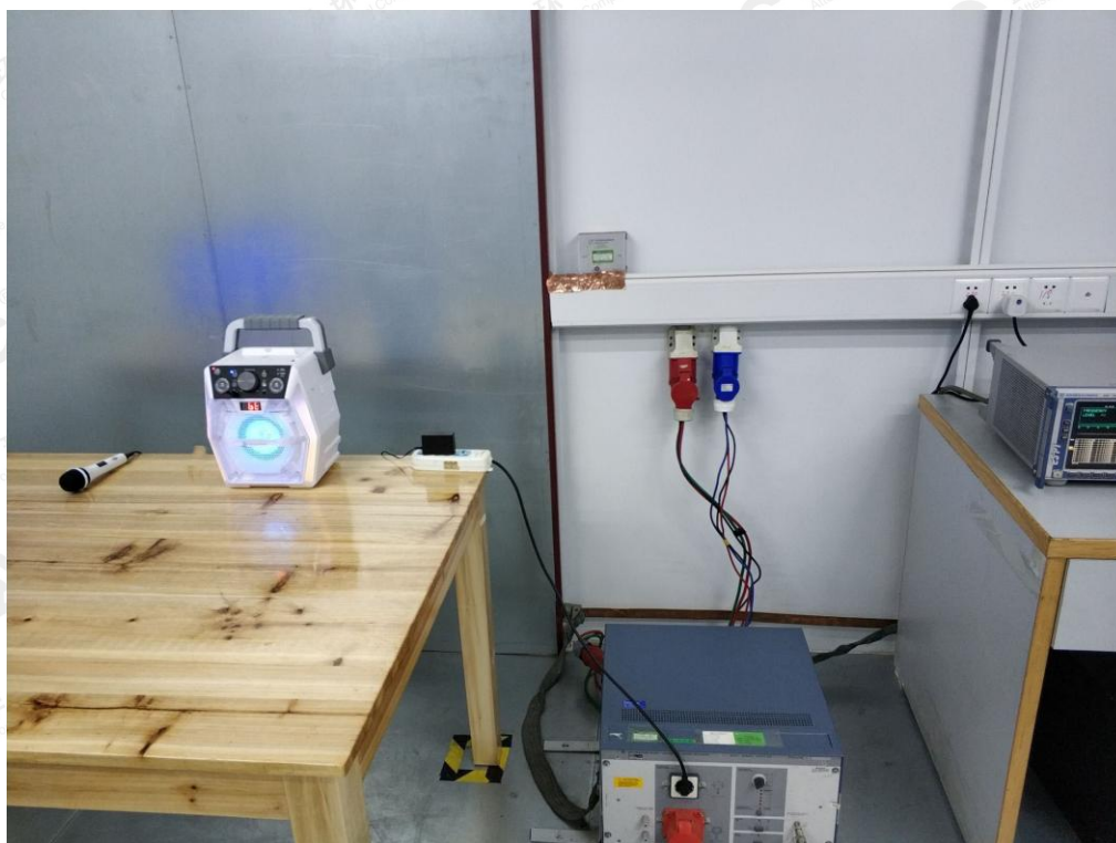
FCC RADIATED EMISSION TEST SETUP
