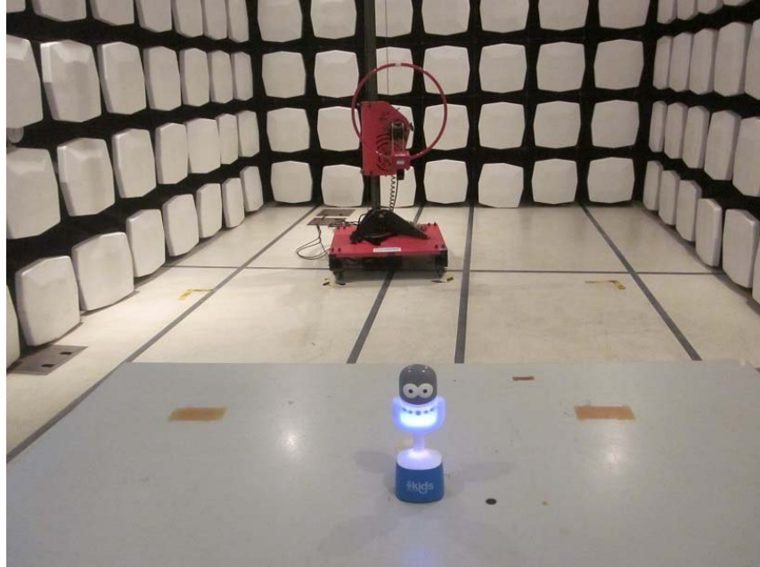
Measurement of Radiated Emission Test Set Up
