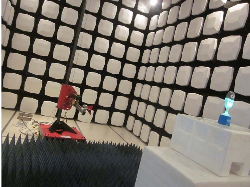
Measurement of Radiated Emission Test Set Up
