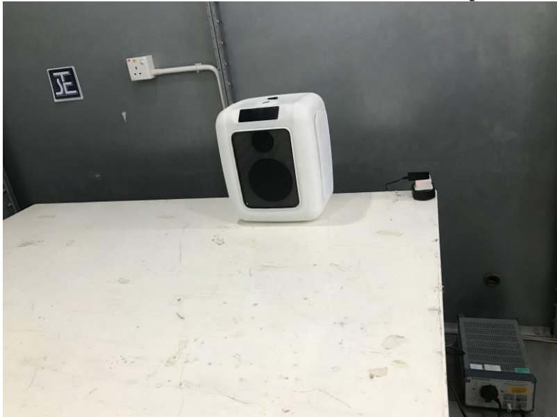
Measurement of Conducted Emission Test Set Up
