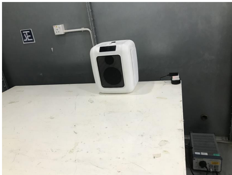
Measurement of Conducted Emission Test Set Up
