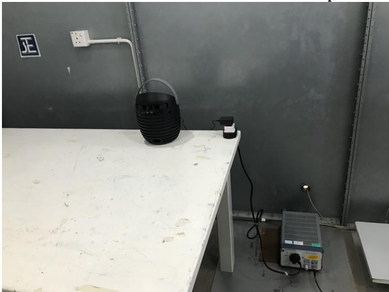
Measurement of Conducted Emission Test Set Up
