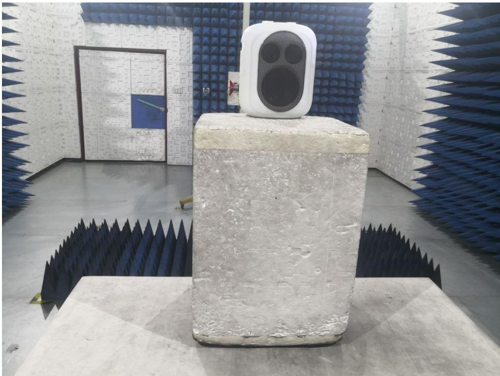
RADIATED EMISSION TEST SETUP ABOVE 1GHz
