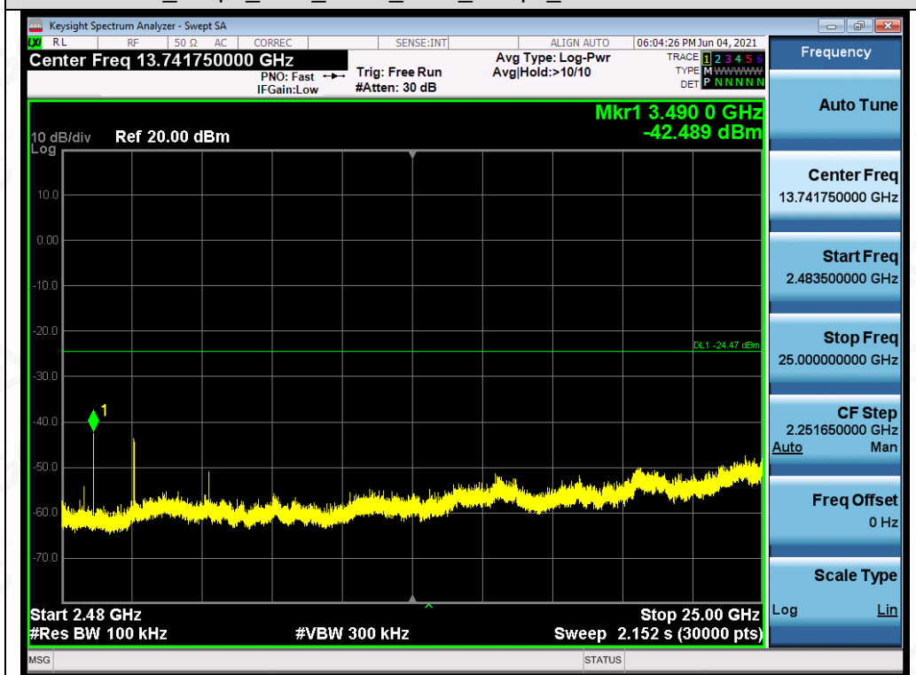
Test_Graph_EDR_ANT1_2402_2Mbps_Higher Band Emissions
