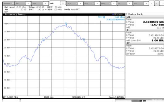
Figure 3. Plot of the 20 dB Channel Bandwidth (Conducted)
