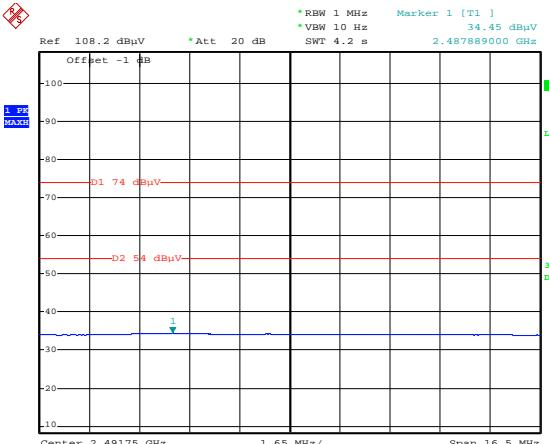
\* offset = Factor (ANT Factor+ Amp Gain + Cable Loss) [dB]
