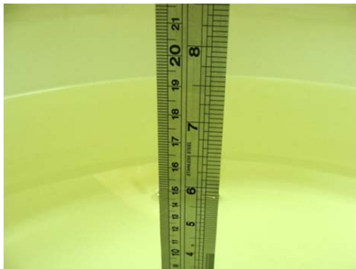
Fig 6.1 Photo of Liquid Height for Body SAR
