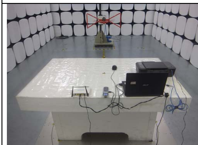
Radiated Emissions Test Setup Below 1GHz
