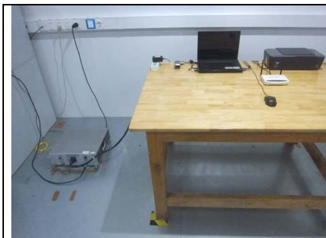
Conducted Emissions Test Setup – Front View
