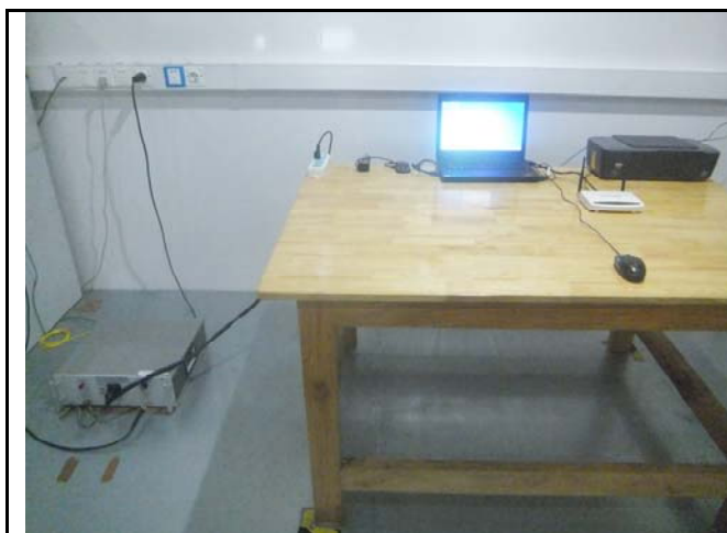
Conducted Emissions Test Setup – Front View
