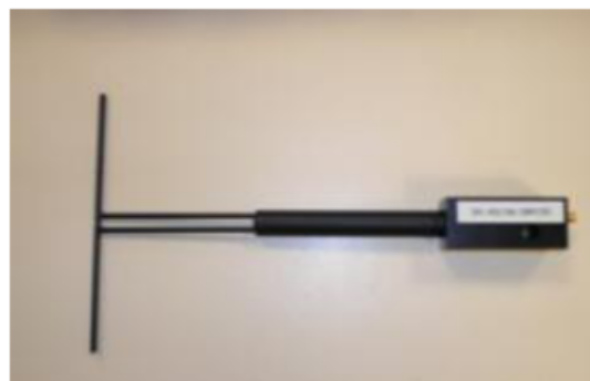
Figure 1 – Satimo COMOSAR Validation Dipole
