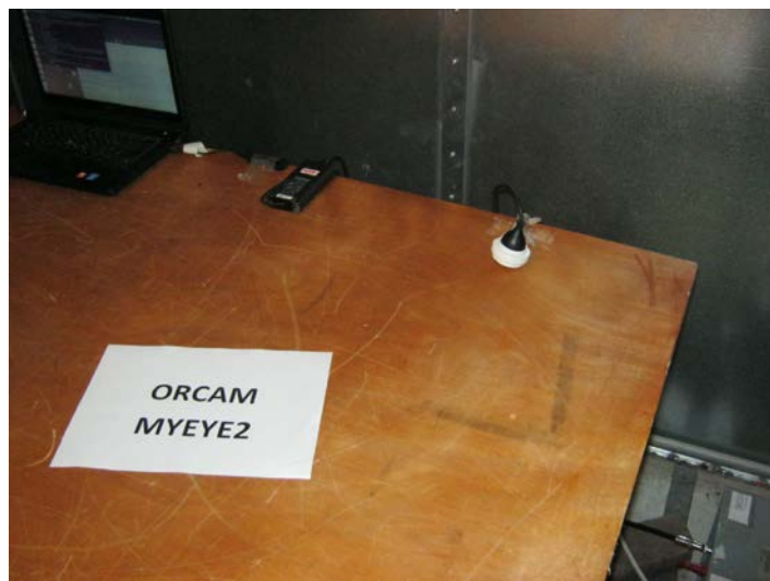
Figure 4. Conducted Emission From AC Mains (Laptop)
