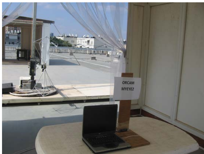
Figure 6. Radiated Emission Test, 30-200MHz
