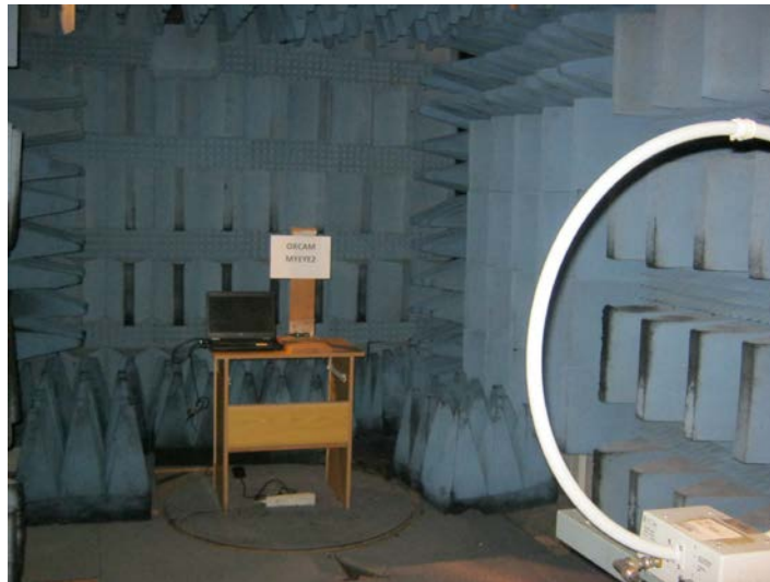
Figure 5. Radiated Emission Test, 0.009-30MHz
