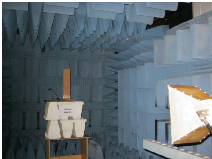
Figure 8. Radiated Emission Test, 1-18GHz
