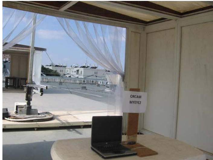
Figure 7. Radiated Emission Test, 200-1000MHz
