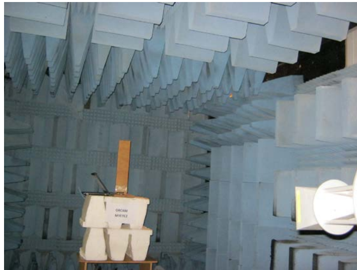
Figure 9. Radiated Emission Test, 18-26.5GHz
