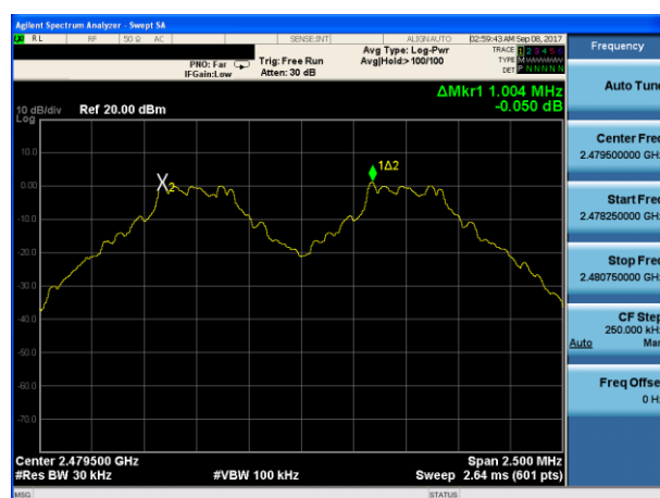
(1Mbps) Channel Separation plot on channel 77-78
