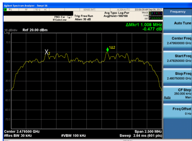
(2Mbps) Channel Separation plot on channel 77-78
