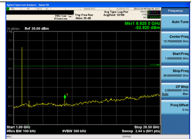
GFSK on channel 78
