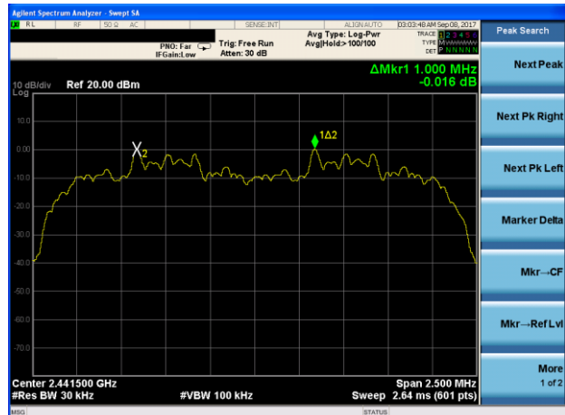
(2Mbps) Channel Separation plot on channel 77-78
