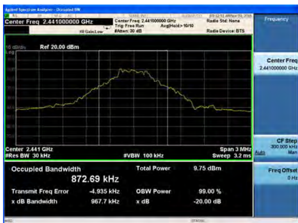
20dB Bandwidth plot on channel 78 (1Mbps)
