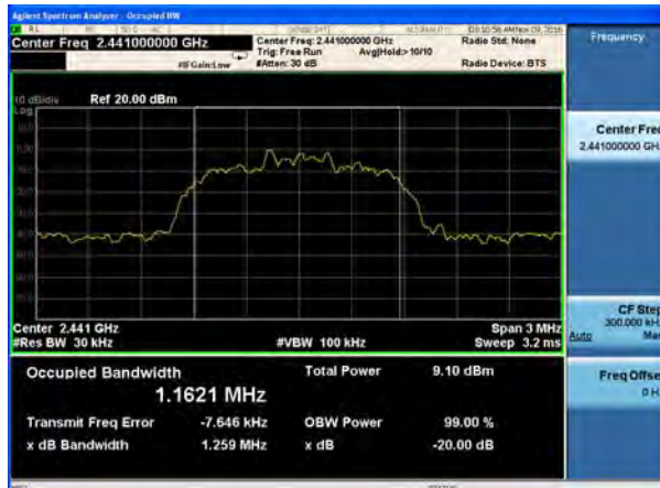
20dB Bandwidth plot on channel 78 (2Mbps)
