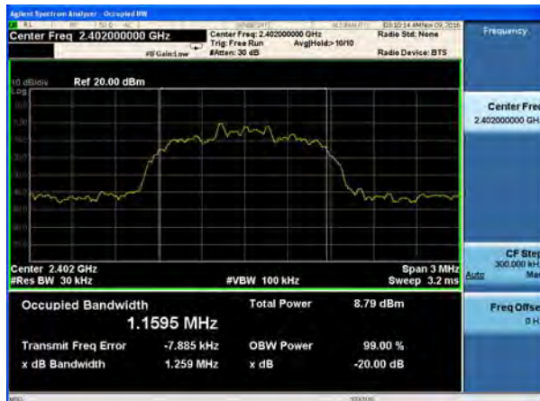
20dB Bandwidth plot on channel 39 (2Mbps)
