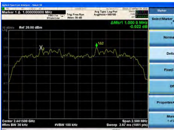
(2Mbps) Channel Separation plot on channel 77-78
