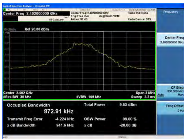
20dB Bandwidth plot on channel 39 (1Mbps)
