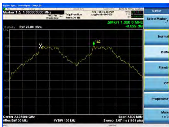
(1Mbps) Channel Separation plot on channel 39-40
