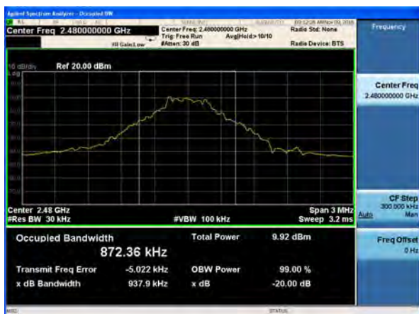
20dB Bandwidth plot on channel 78 (1Mbps)
