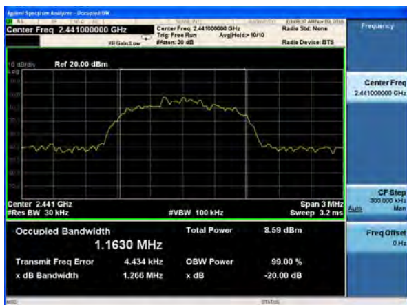
20dB Bandwidth plot on channel 78 (3Mbps)
