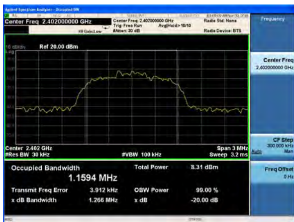
20dB Bandwidth plot on channel 39 (3Mbps)
