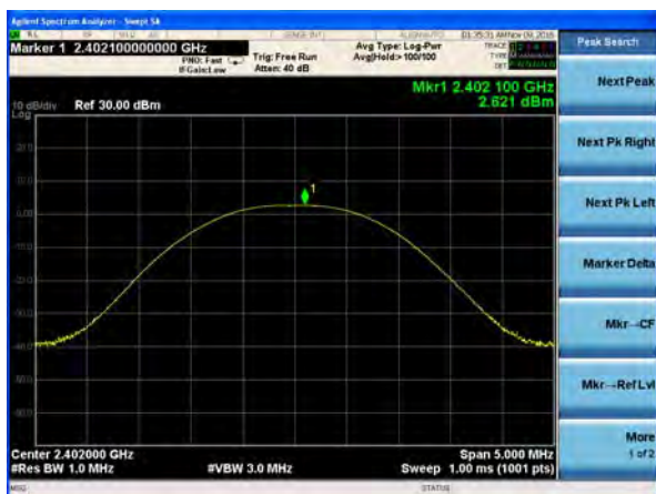
Peak output Power plot on channel 39 (1Mbps)
