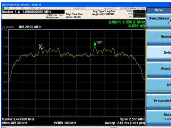
(2Mbps) Channel Separation plot on channel 77-78
