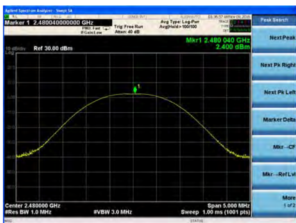
Peak output Power plot on channel 78 (1Mbps)
