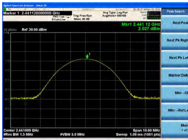
Peak output Power plot on channel 78 (2Mbps)
