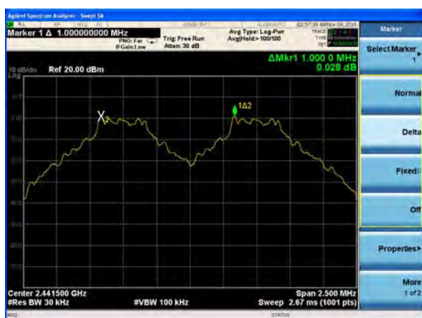
(1Mbps) Channel Separation plot on channel 77-78
