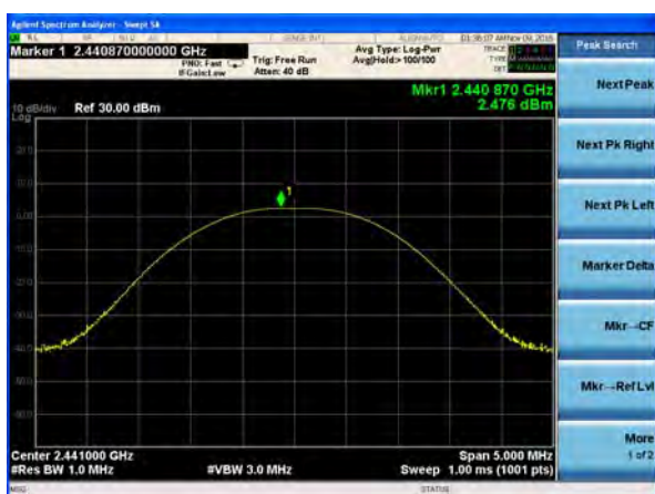
Peak output Power plot on channel 78 (1Mbps)
