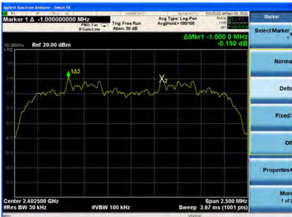
(2Mbps) Channel Separation plot on channel 39-40
