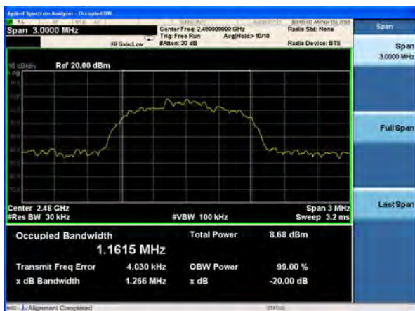
20dB Bandwidth plot on channel 78 (3Mbps)
