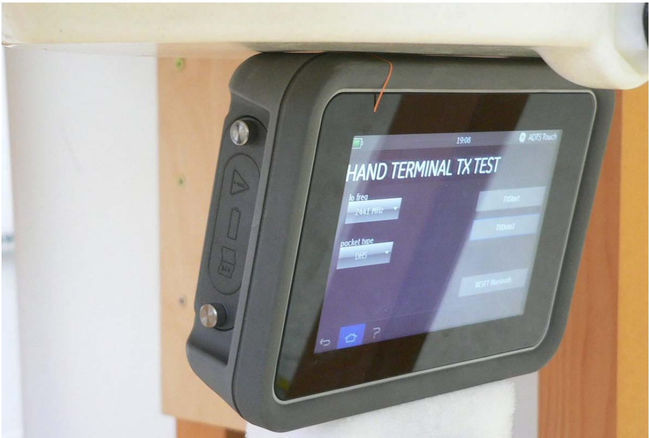
Fig. 11: Body supported configuration, position 3, top edge toward the phantom, gap = 0 mm.
