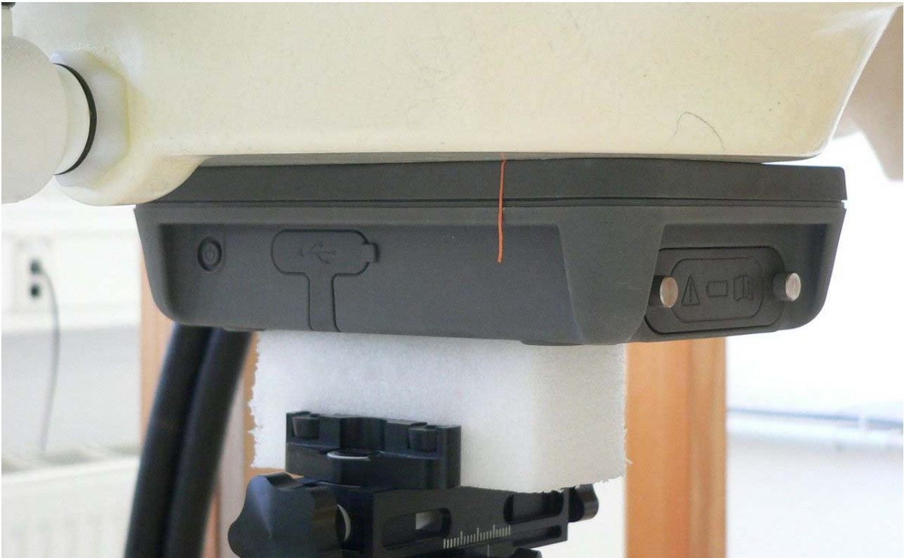
Fig. 9: Body supported configuration, position 1, front side toward the phantom, gap = 0 mm.
