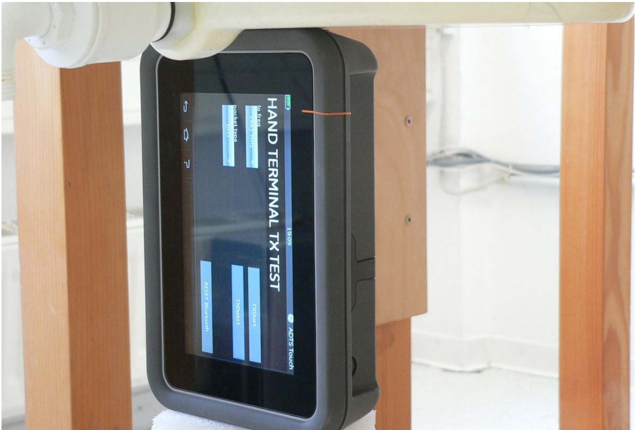
Fig. 12: Body supported configuration, position 4, right edge toward the phantom, gap = 0 mm.
