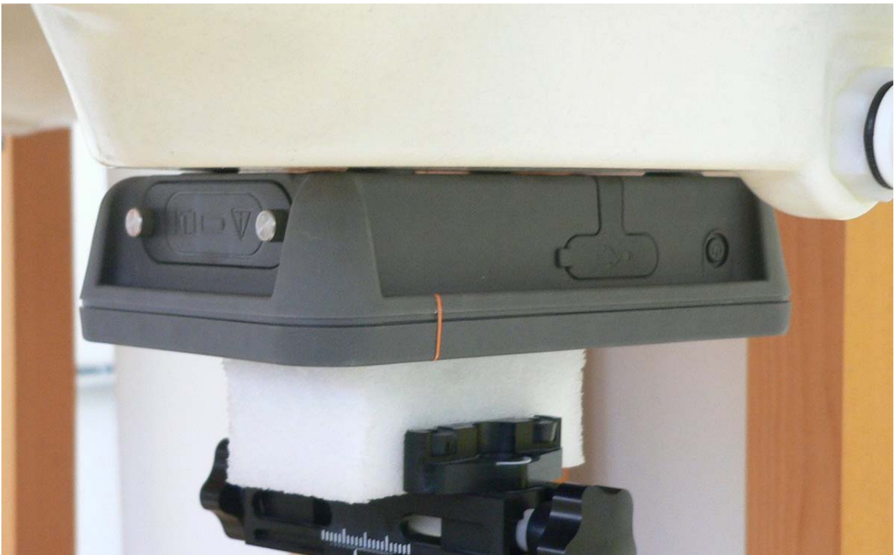
Fig. 10: Body supported configuration, position 2, back side toward the phantom, gap = 0 mm.
