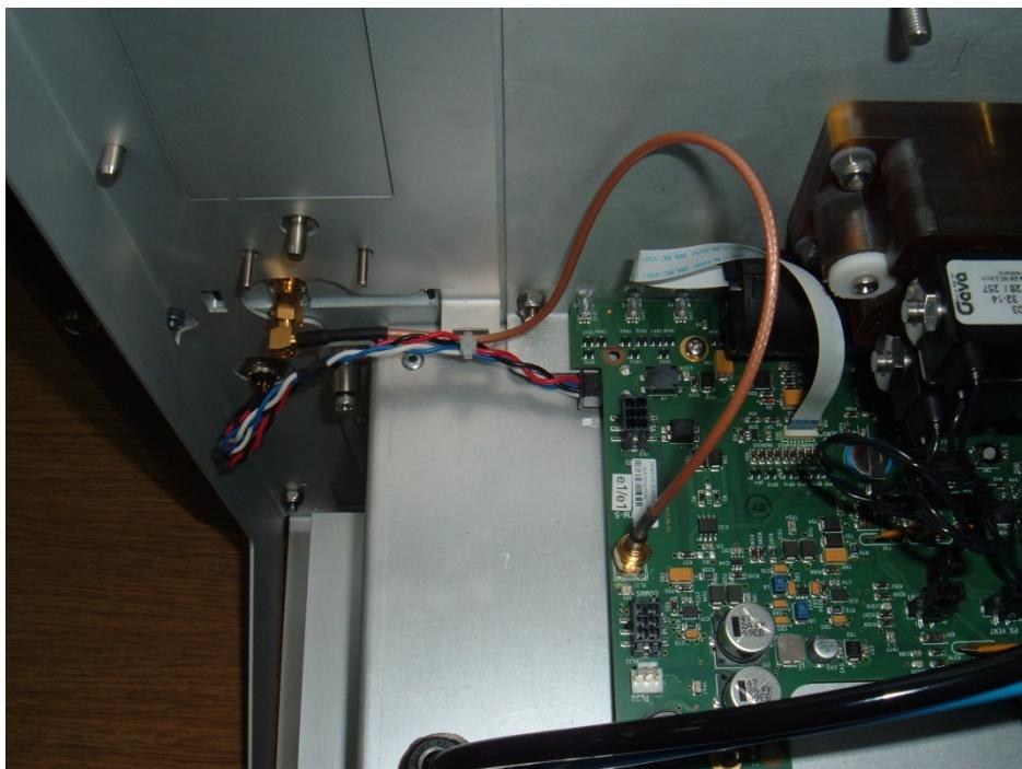
PCB Top Side – SMA Antenna Connector to Right
