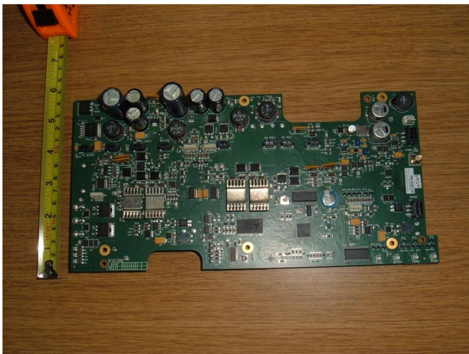
PCB Underside – Wireless Module to Left
