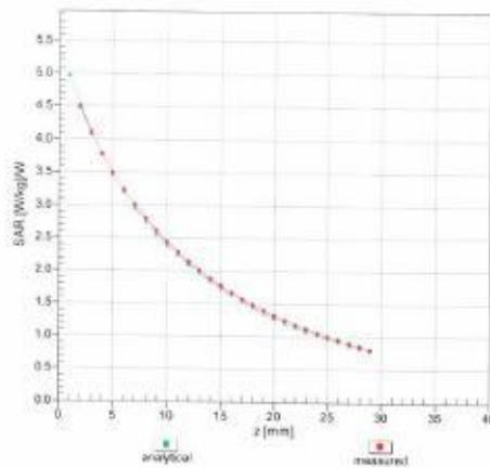
$f = 450 \text{ MHz}, \text{WGLS Flat Phantom 4.4}$
