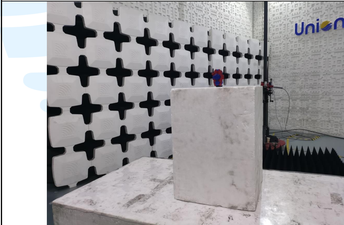
Radiated emission Test Setup (Above 1 GHz)
