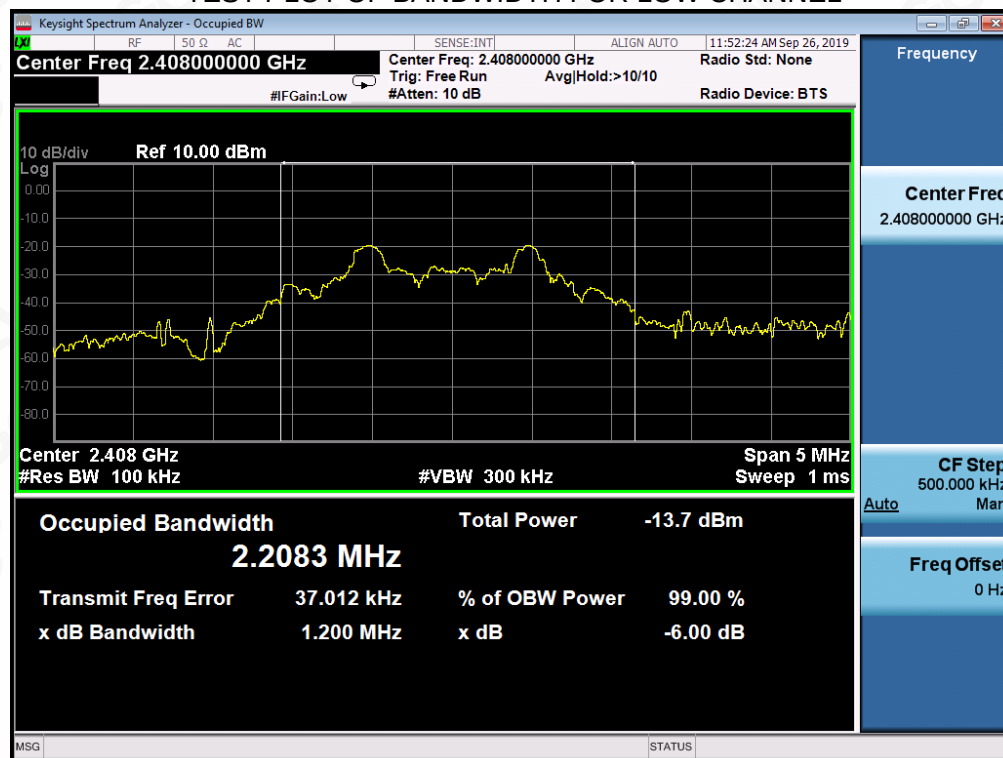
TEST PLOT OF BANDWIDTH FOR LOW CHANNEL
