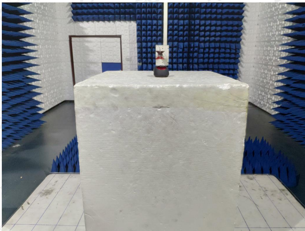
FCC RADIATED EMISSION TEST SETUP ABOVE 1GHZ
