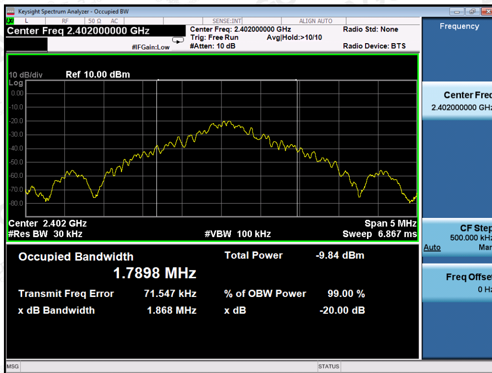
TEST PLOT OF BANDWIDTH FOR LOW CHANNEL
