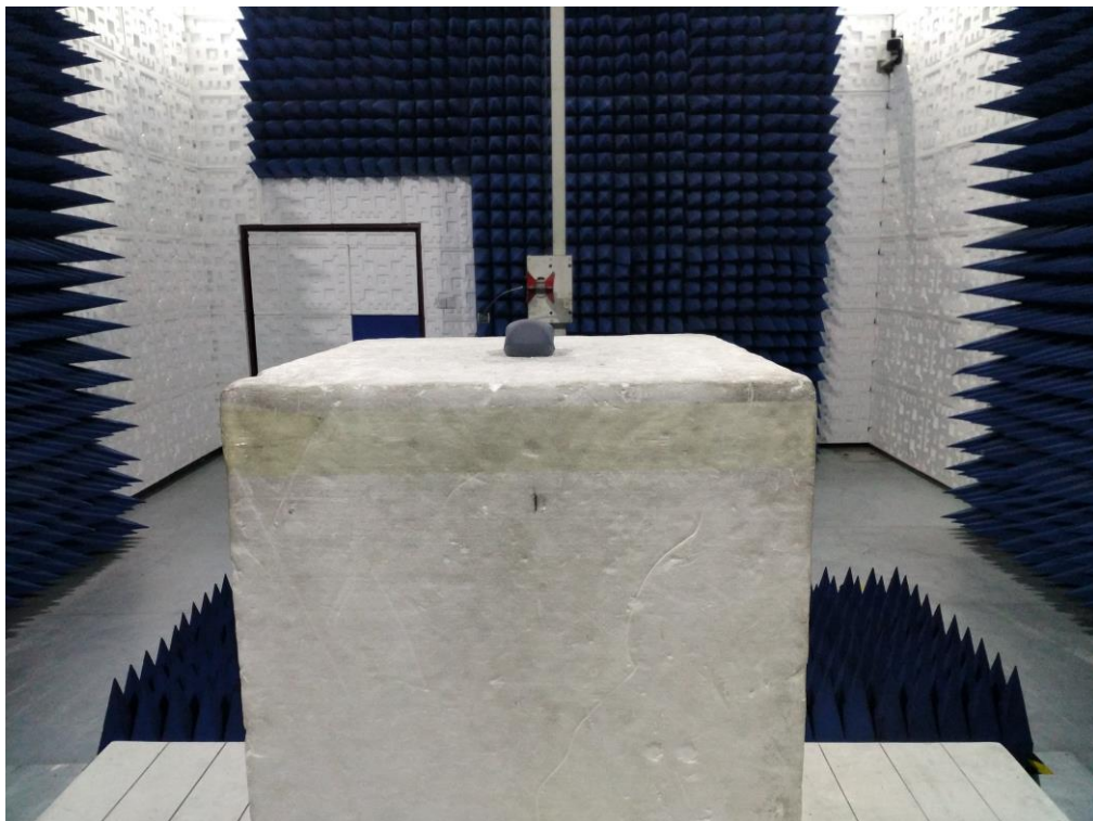
FCC RADIATED EMISSION TEST SETUP ABOVE 1GHZ
