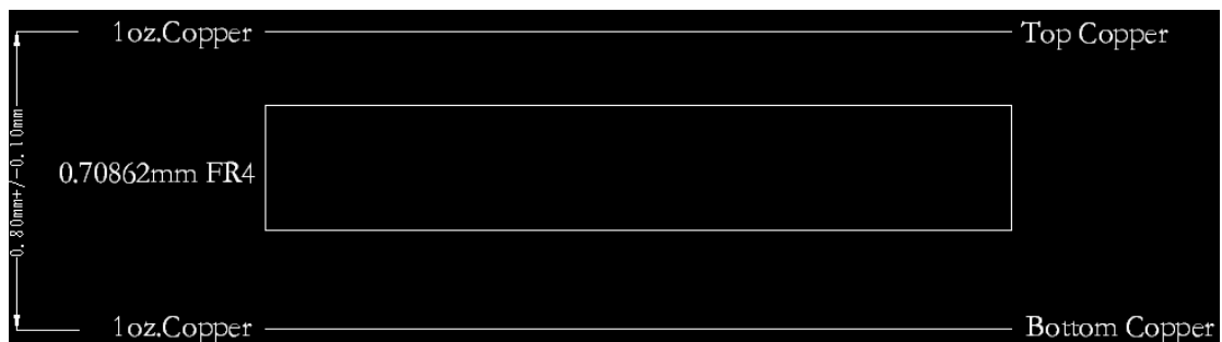
FIGURE 10 PCB LAYER STACK UP
