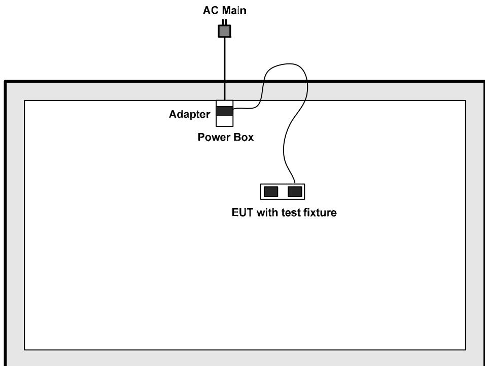
**Test Setup Diagram - Radiated Test (30MHz~1GHz)**
