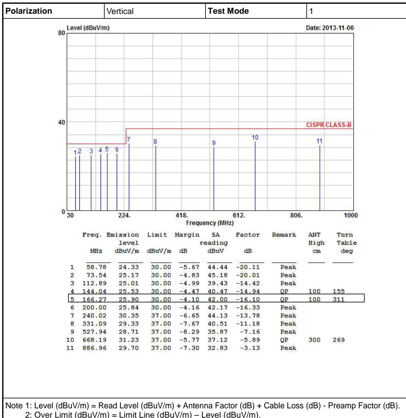
Note 1: Level (dBuV/m) = Read Level (dBuV/m) + Antenna Factor (dB) + Cable Loss (dB) - Preamplifier Factor (dB).
