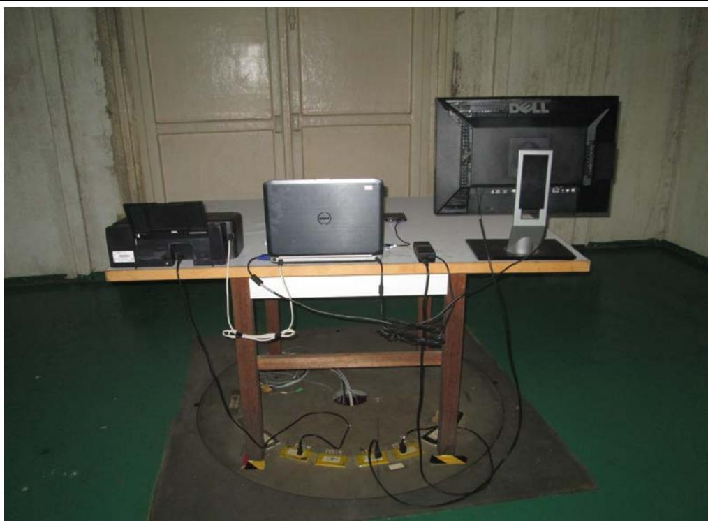
**Radiated Emission Above 1GHz Test**
