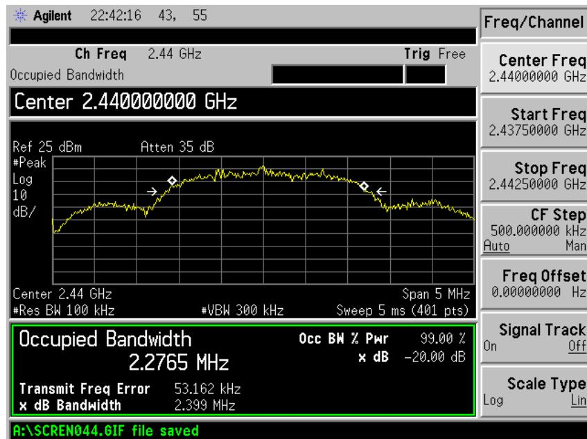
Result data graph shows 20 dB bandwidth of Highest Channel, BW = 2.449MHz
