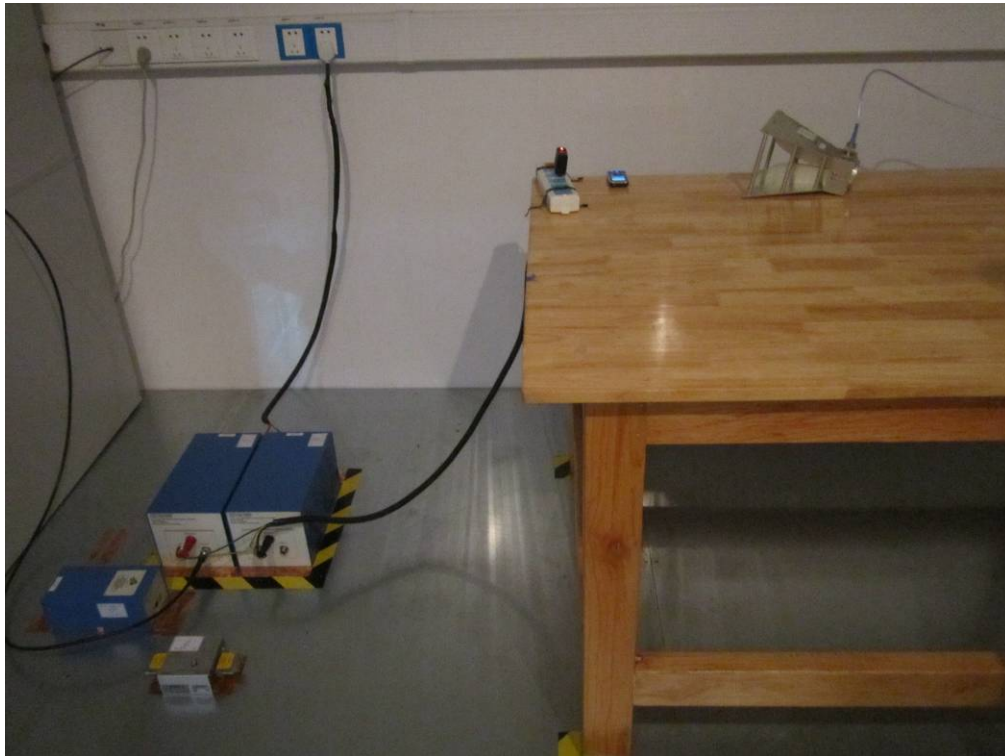
Conducted Emissions Test Setup Front View
