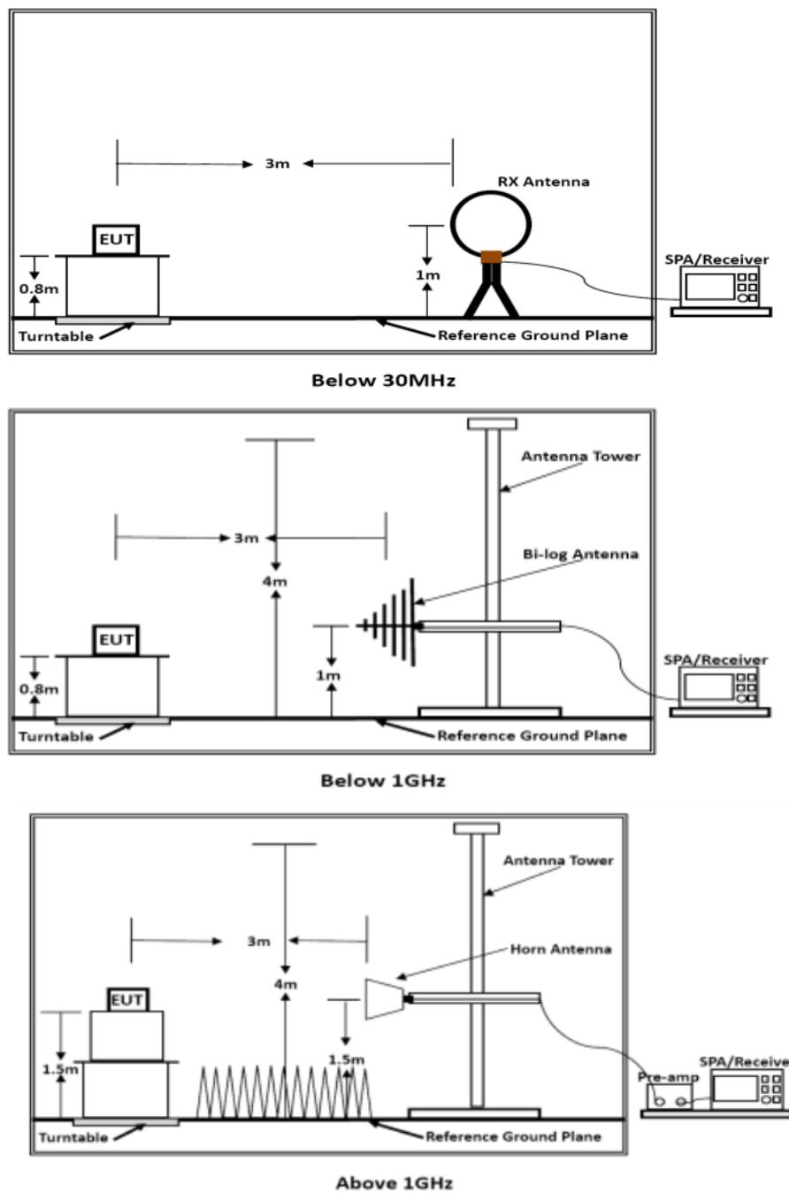
Above 18 GHz shall be extrapolated to the specified distance using an extrapolation factor of 20 dB/decade from 3m to 1m.
