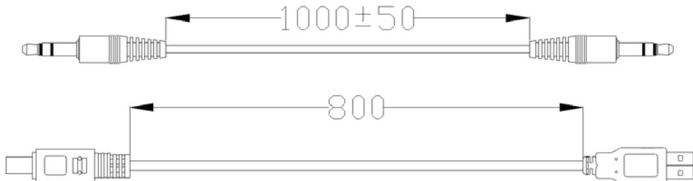
**1. OD3.5 to OD3.5 black audio extending cable****2. USB A to Mini USB 5Pin connector**
