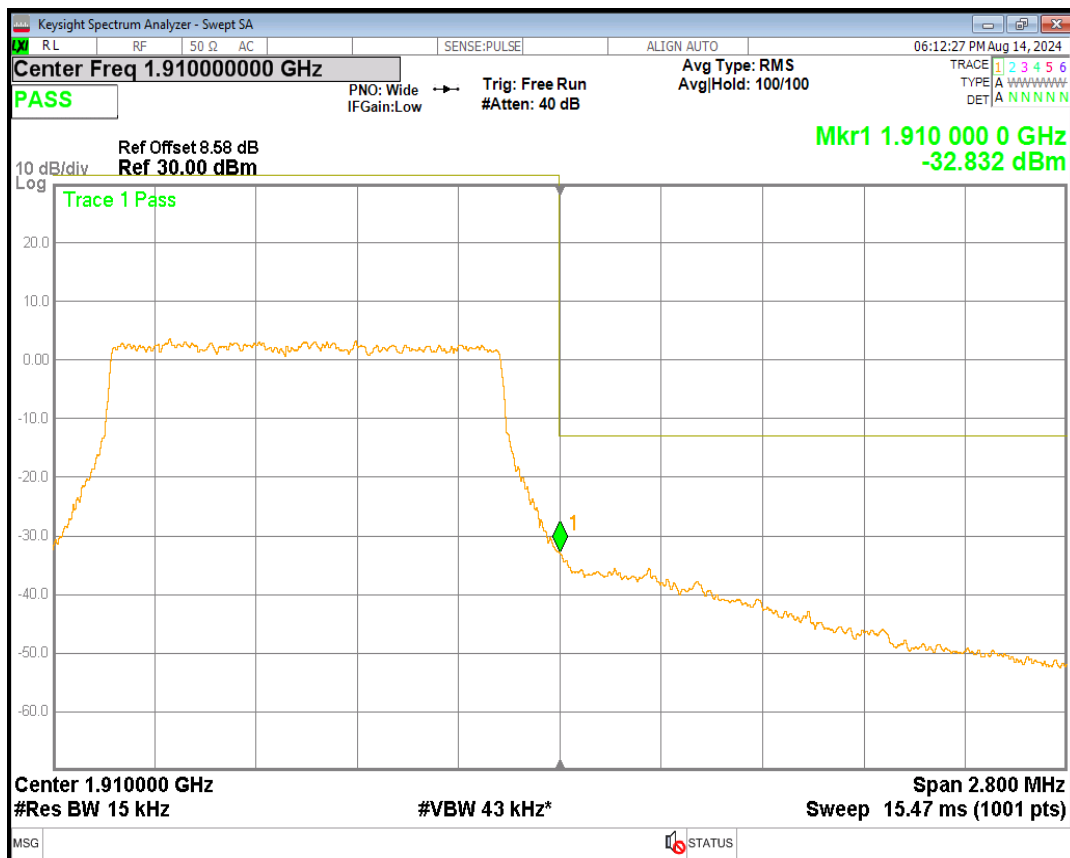
Band2 16QAM BW=3MHz Channel=18615 RB Size=15 Position=#0
