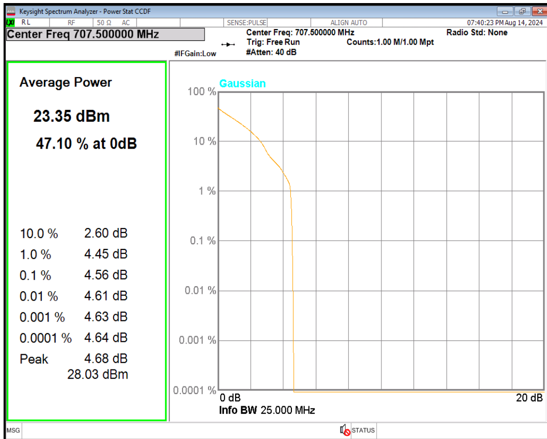
Band12 QPSK BW=10MHz Channel=23130 RB Size=1 Position=#0
