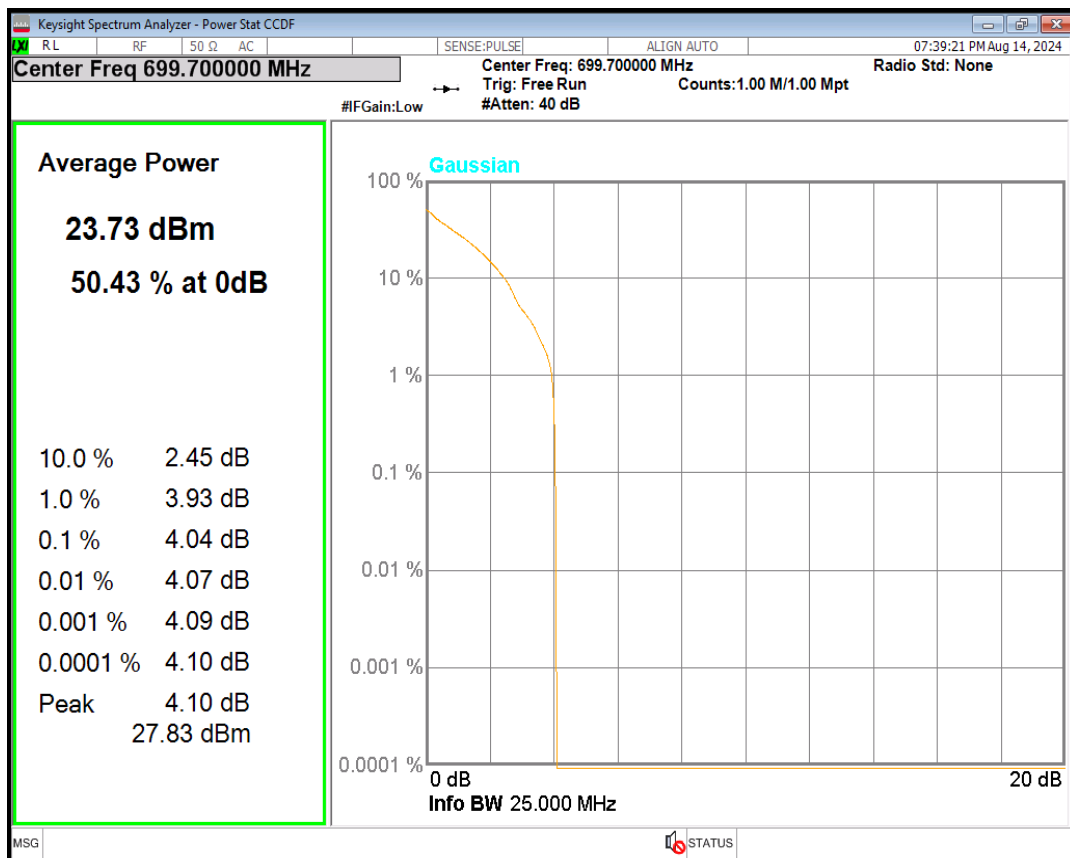
Band12 16QAM BW=5MHz Channel=23095 RB Size=1 Position=#0
