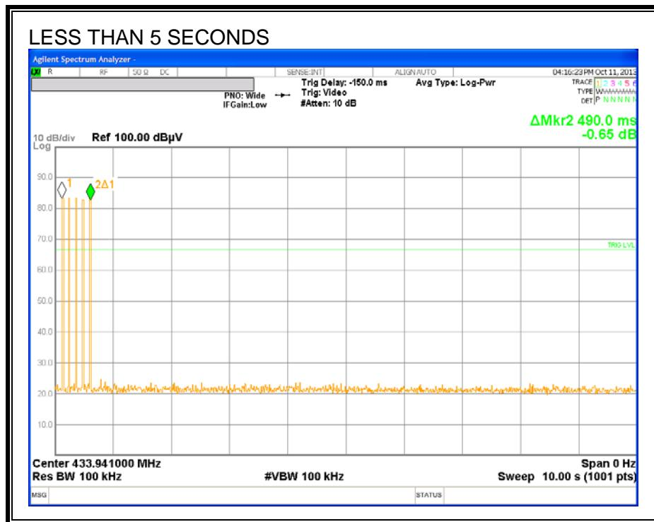
EUT automatically shuts off within 0.5s.
