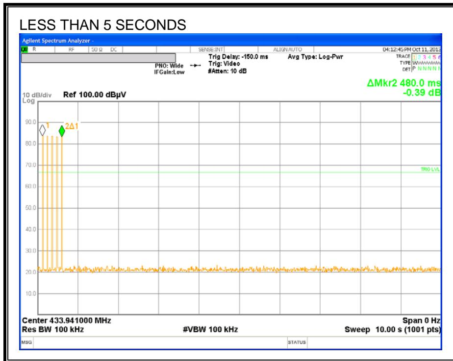
EUT automatically shuts off within 0.5s.
