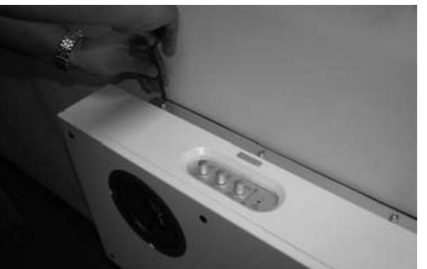
19 Secure bottom bracket with the two 50 mm long cap head hardware provided from the bottom side of the bracket.
