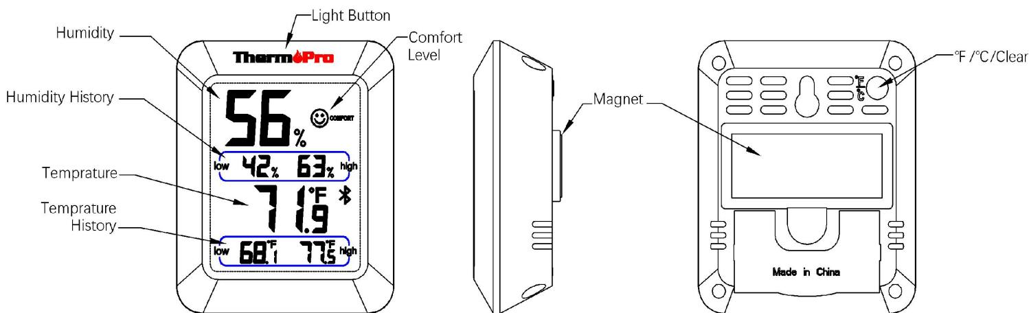
1. Display: Displays the current humidity and temperature, maximum and minimum humidity/temperature recorded in the past
