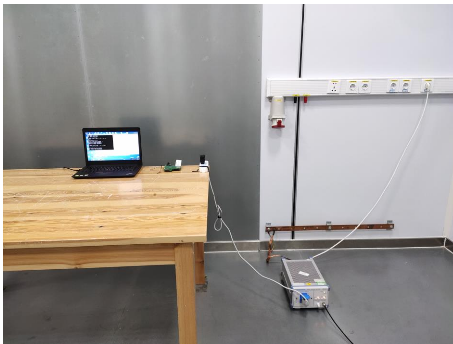
Fig. 4 Power line conducted emission setup photo
