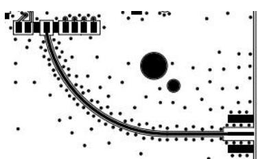
The line between the External antenna and the BT module must be 50 ohm.
