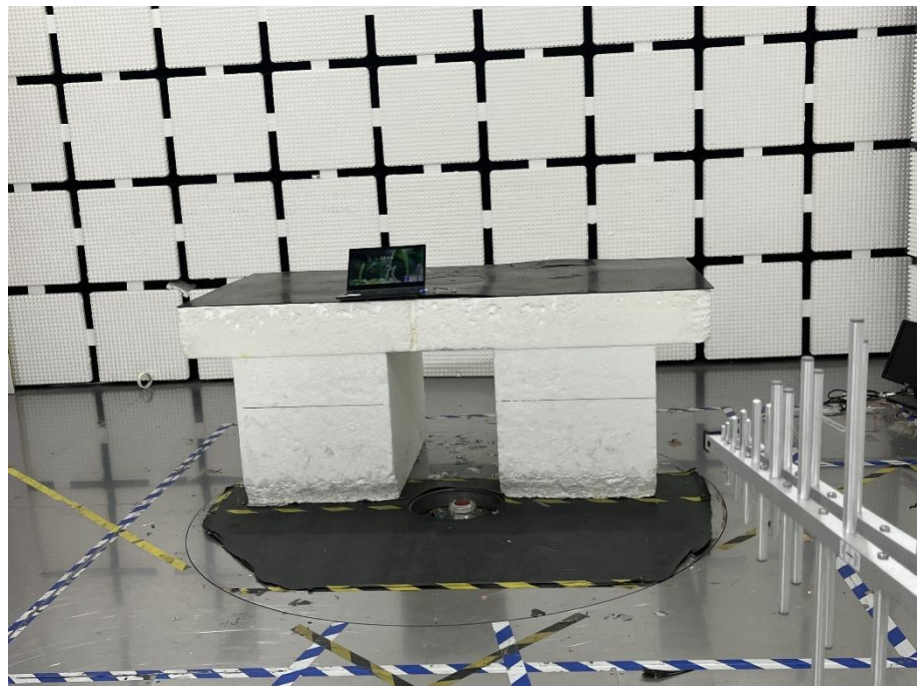
Radiation Emission Test Setup (30MHz to 1GHz)
