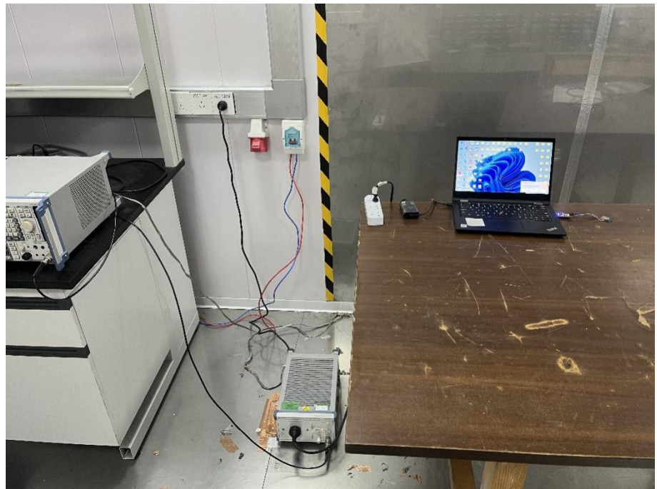
Conducted Emission Test Setup
