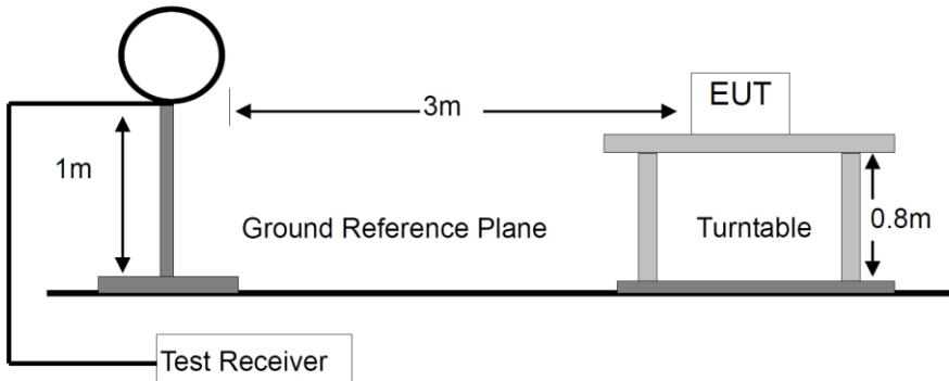
For Radiated Emission 30-1000MHz
