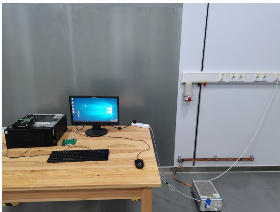
Fig. 4 Power line conducted emission setup photo
