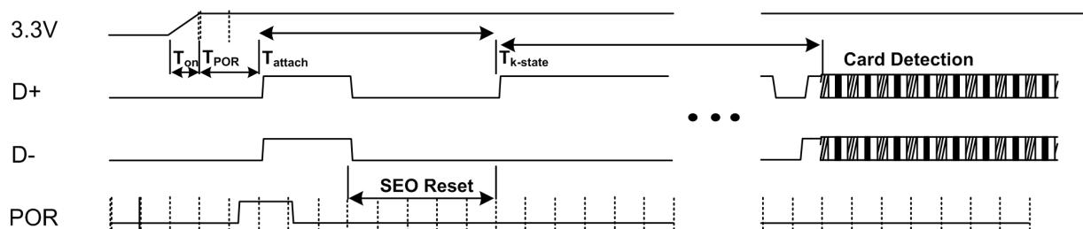
**T<sub>on</sub>:** The main power ramp up duration
