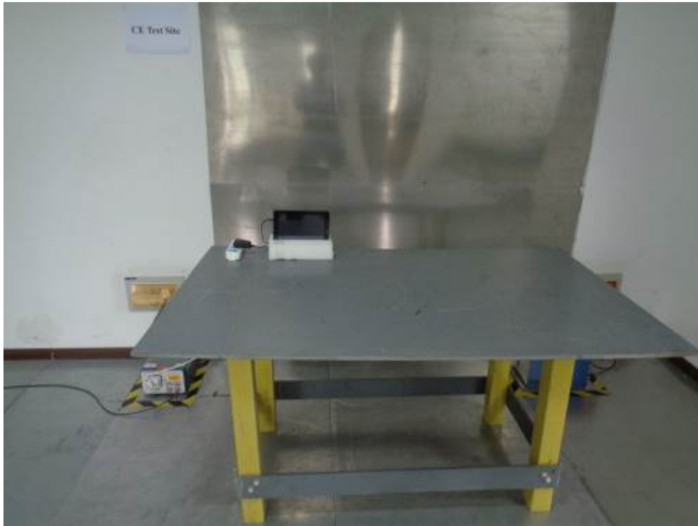
Conducted Emissions Test Setup Front View
