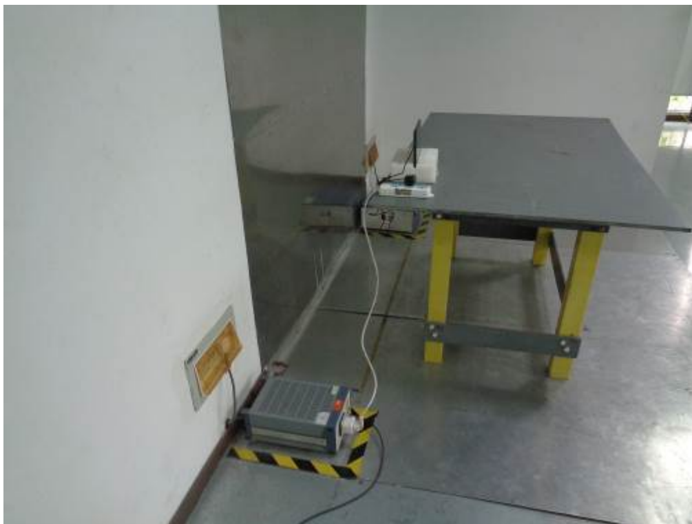
Conducted Emissions Test Setup Side View
