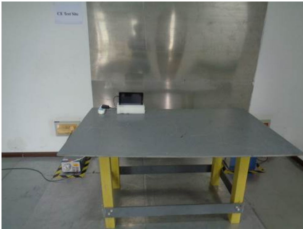
Conducted Emissions Test Setup – Front View
