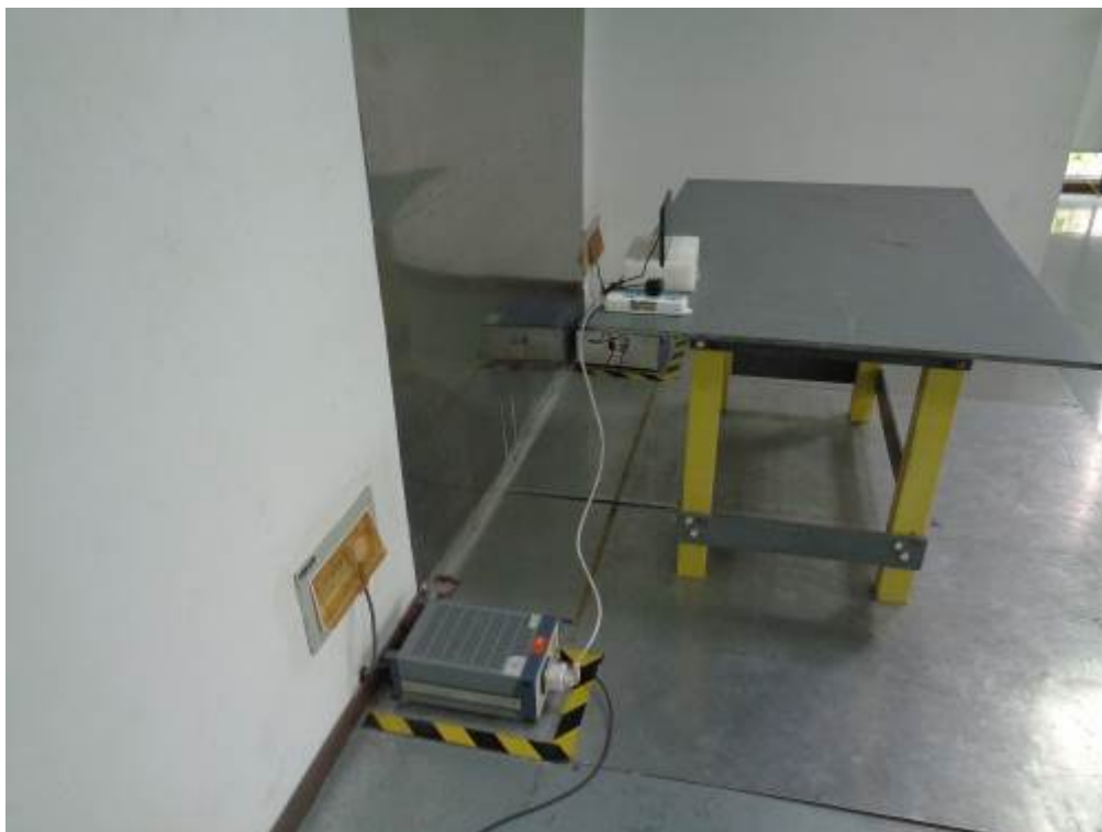
Conducted Emissions Test Setup – Side View
