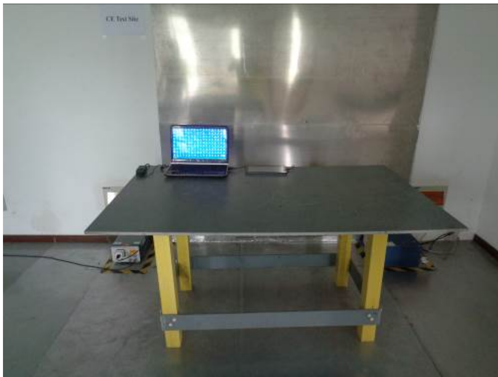
Conducted Emissions Test Setup Front View
