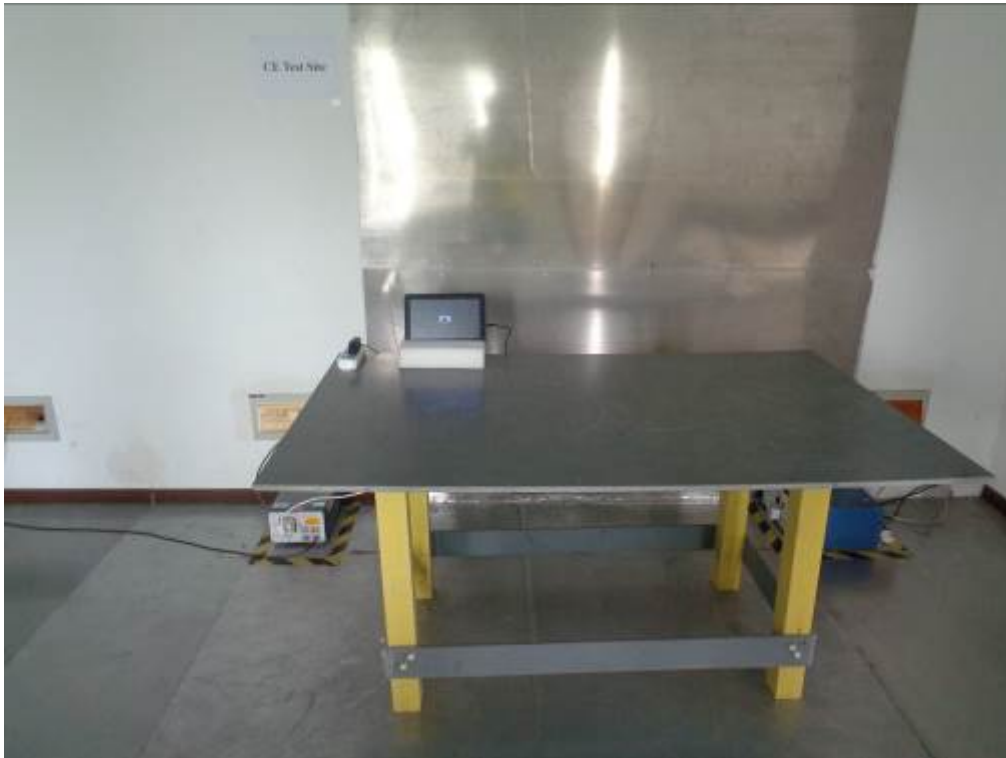
Conducted Emissions Test Setup – Front View
