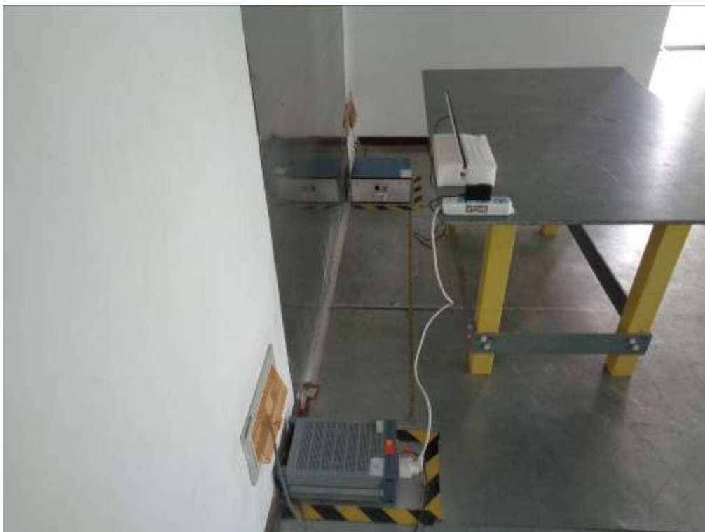
Conducted Emissions Test Setup – Side View
