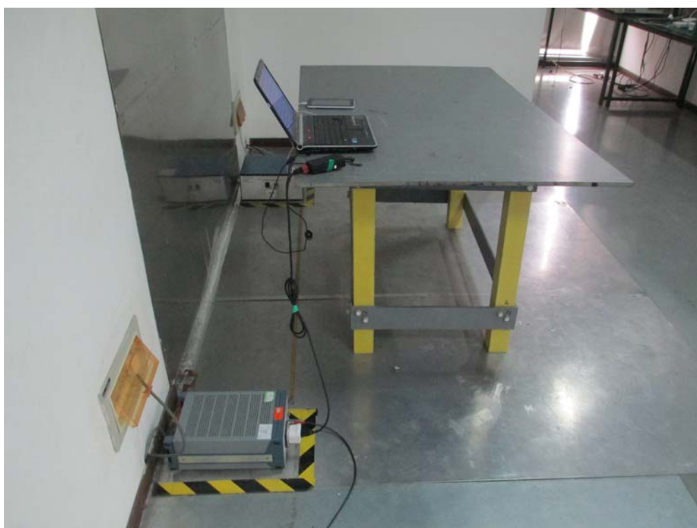
Conducted Emissions Test Setup Side View
