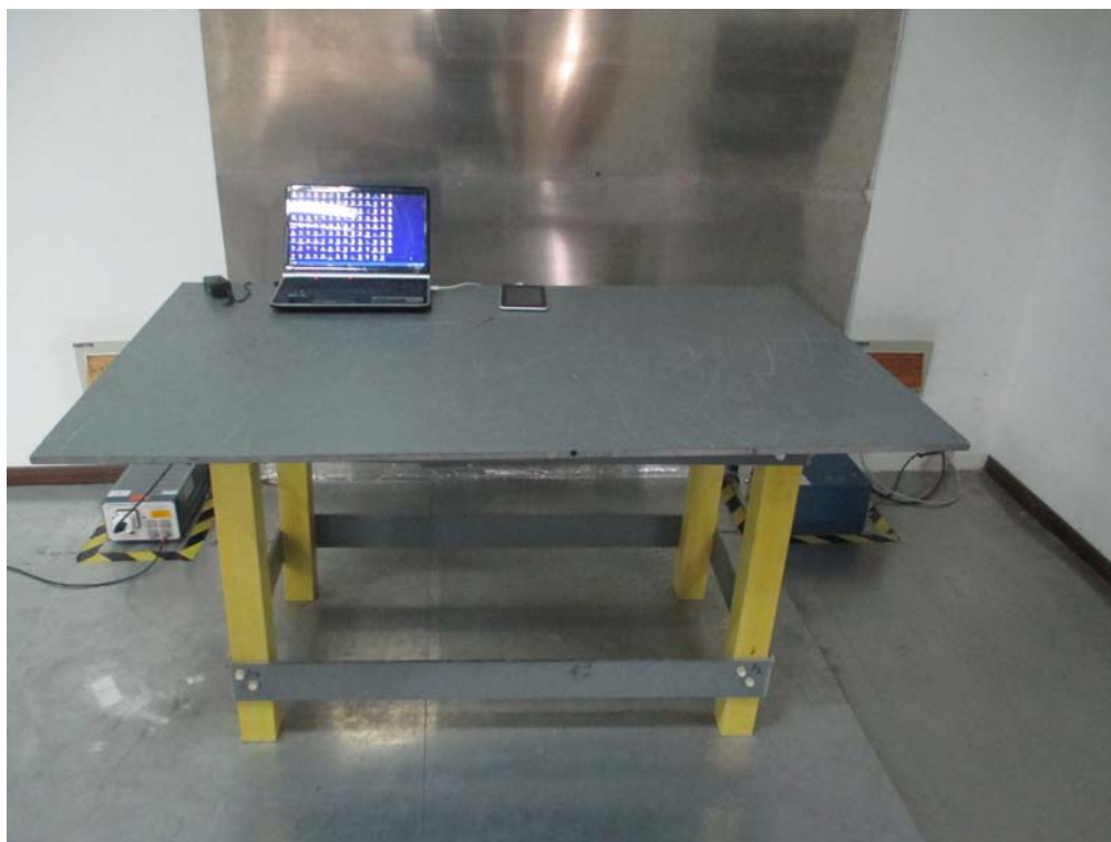
Conducted Emissions Test Setup Front View
