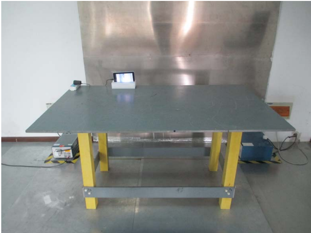
Conducted Emissions Test Setup Front View
