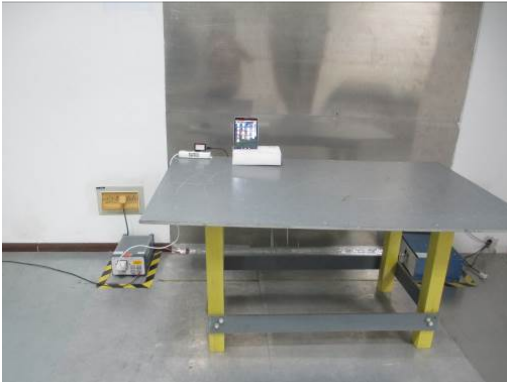
Conducted Emissions Test Setup – Front View
